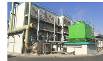
Figure: Sanyou's equipment for the disposal of low-concentration waste gas through the biochemical process
